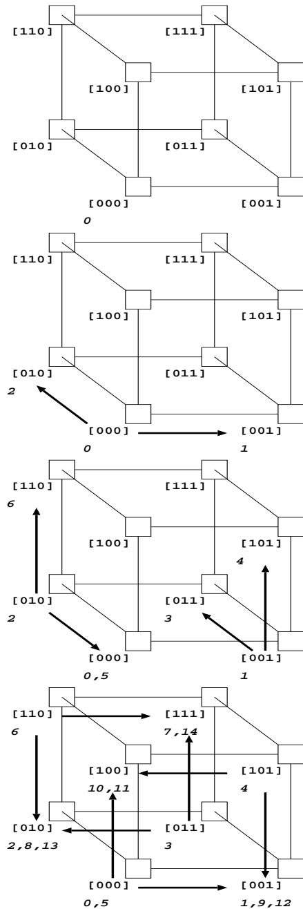
Figure 21. Step by step illustration of load balanced parent-child mapping
