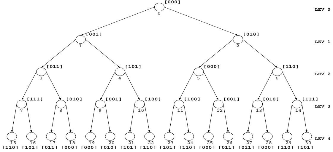
Figure 20. Adjacent parent-child mapping with round robin rotation; allocated hypercube node numbers are shown within square brackets
