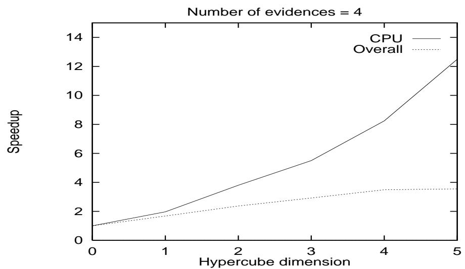
Figure 31. Speedup vs Cube dimension for a tree of 50 nodes
