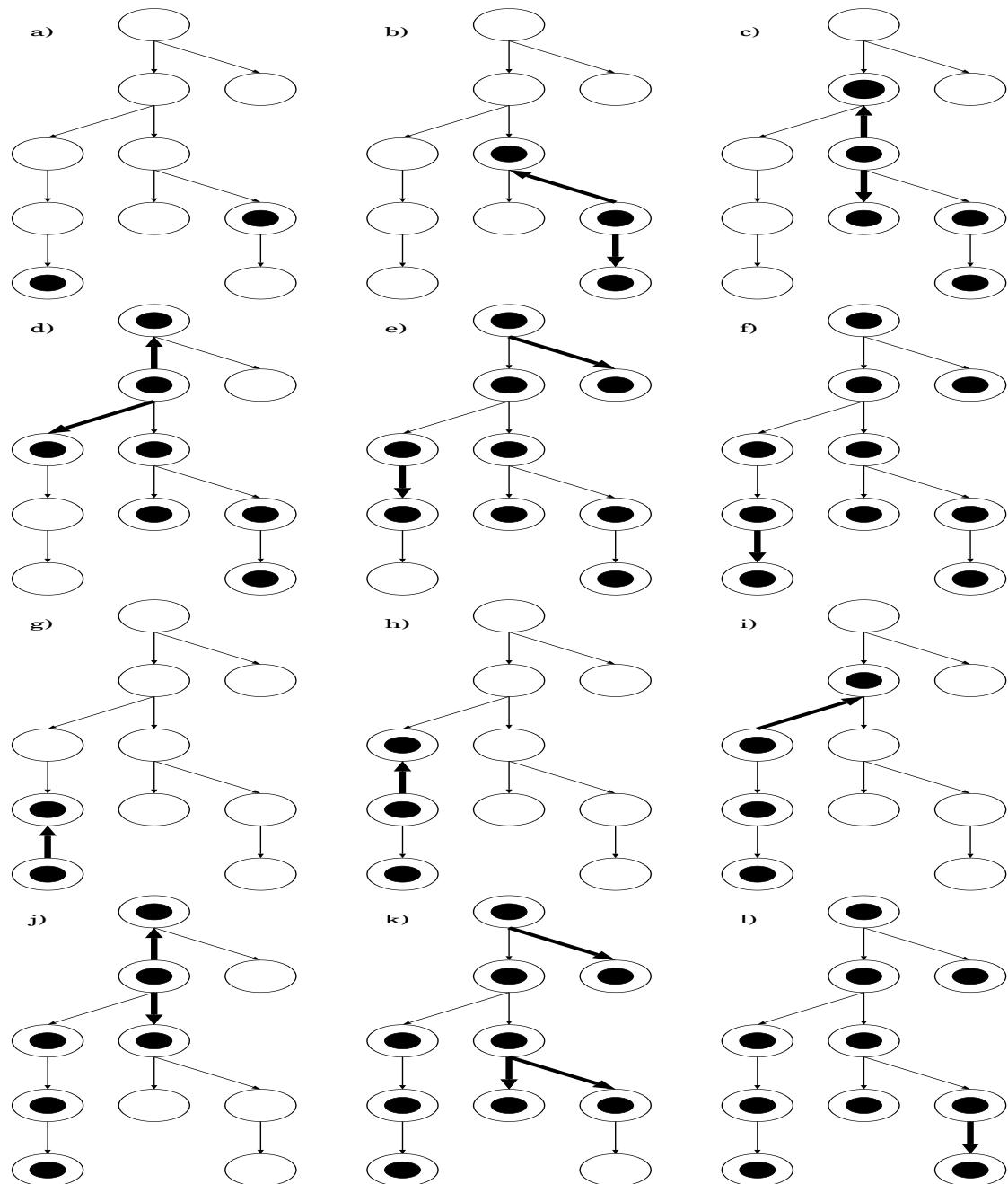
Figure 12. Polytree algorithm : separate phases of network updation for each evidence
