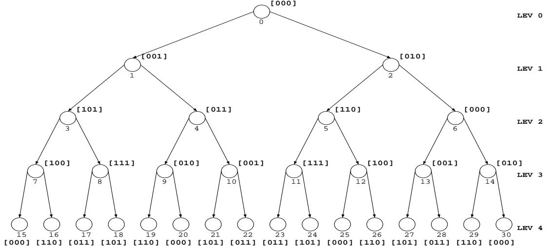
Figure 19. Adjacent parent-child mapping with alternate bit reversal; allocated hypercube node numbers are shown within square brackets
