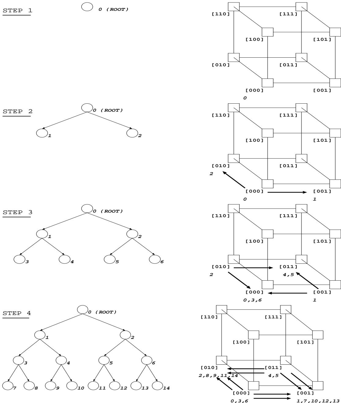
Figure 18. Step by step illustration of parent-child mapping
