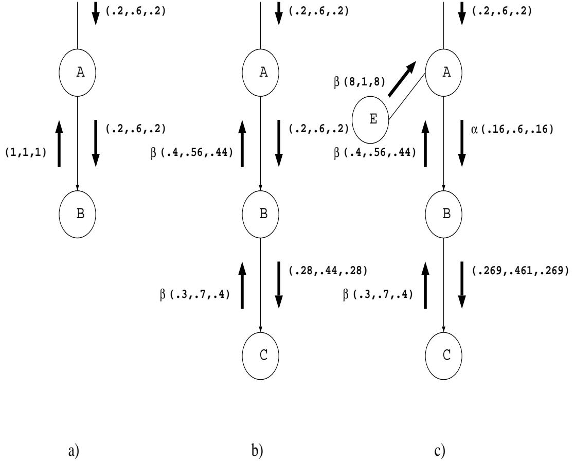
Figure 3. Belief updating and propagation (a) Without check results, (b) With check results C, (c) With evidence E
