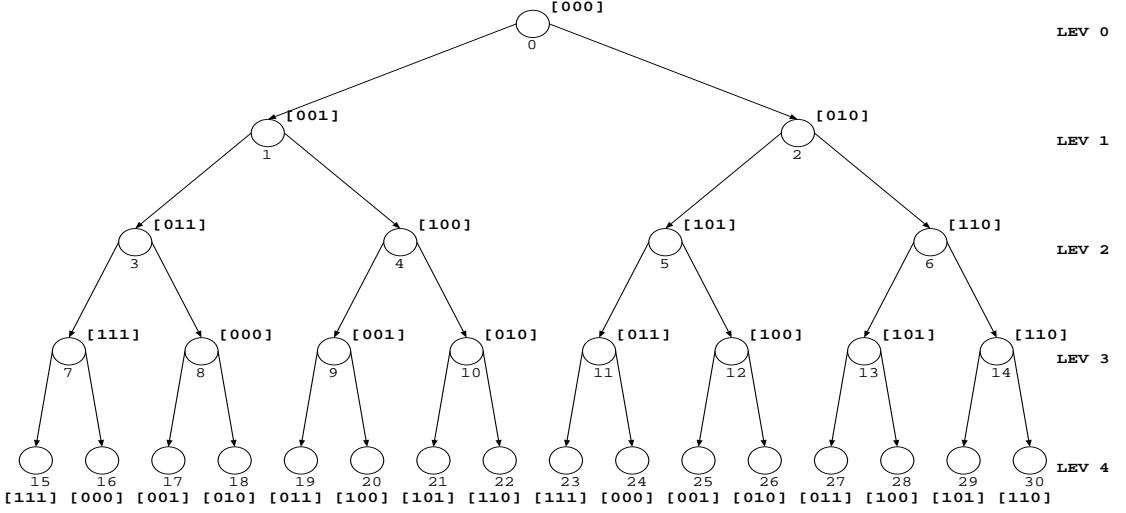
Figure 16. Breadth first mapping; allocated hypercube node numbers are shown within square brackets
