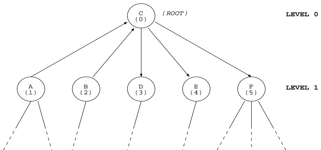
Figure 15. Conversion of the Bayesian tree to a levelled single-parent tree, with node C as the pivot
