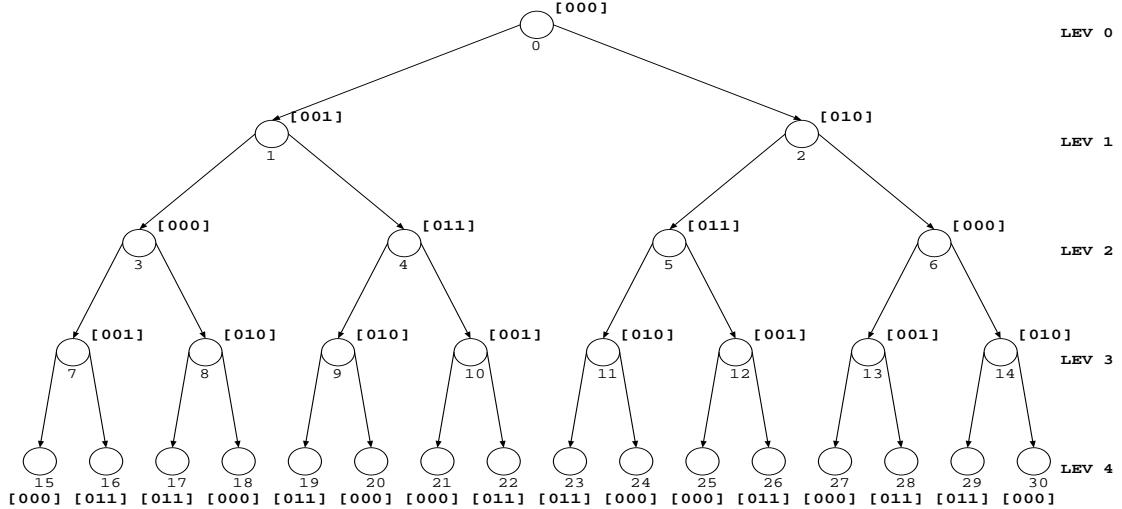
Figure 17. Adjacent parent-child mapping; allocated hypercube node numbers are shown within square brackets
