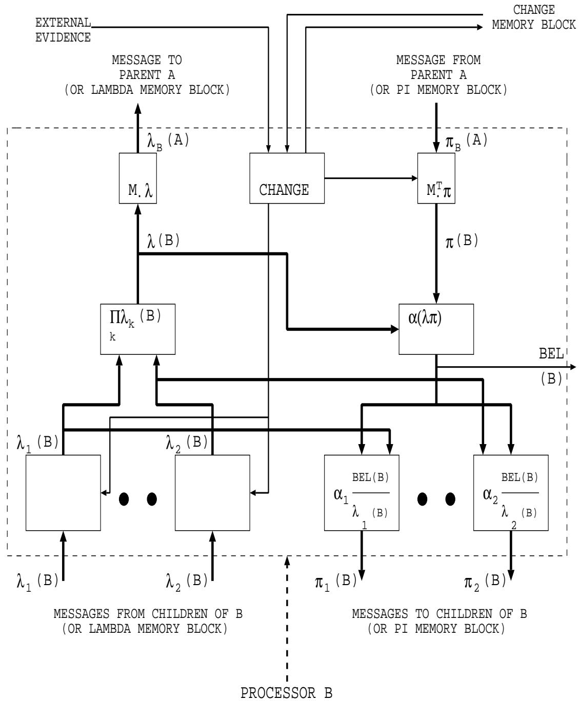
Figure 25. The structure of a single Bayesian node [39]
