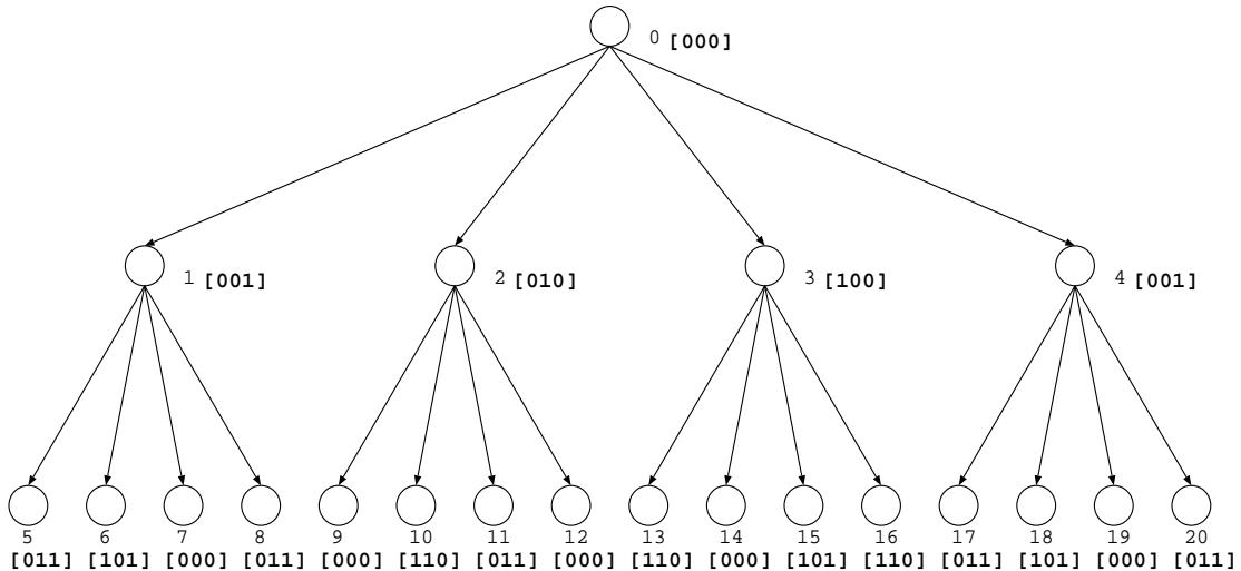
Figure 24. Round robin rotation in a quarternary tree; allocated hypercube node numbers are shown within square brackets
