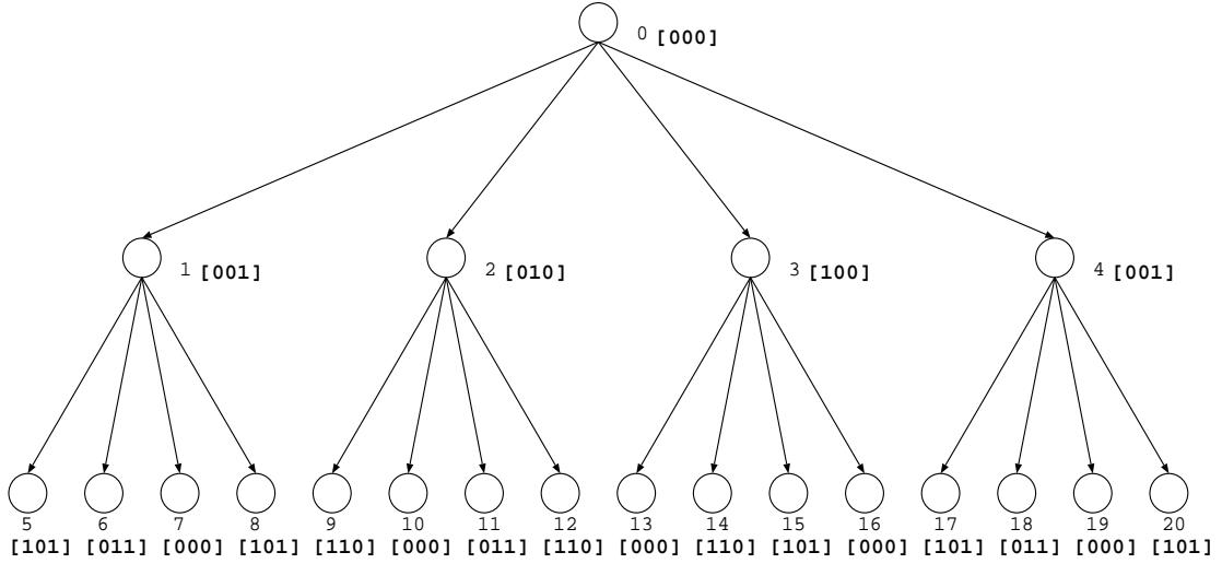
Figure 23. Alternate bit reversal in a quarternary tree; allocated hypercube node numbers are shown within square brackets
