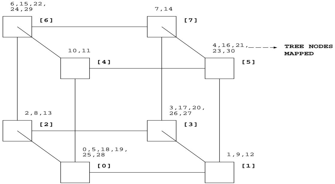
Figure 22. Hypercube showing round robin mapping of a complete binary tree of height 4
