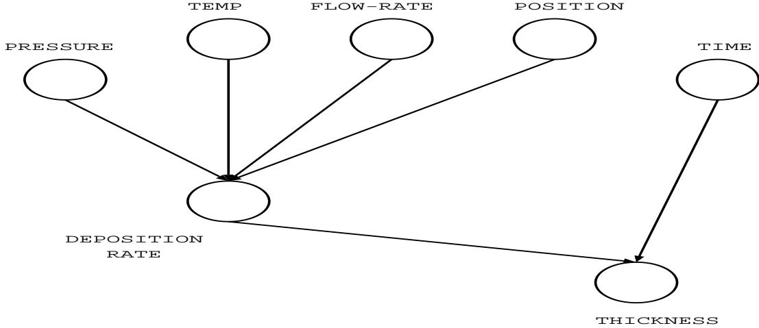
Figure 7. Bayesian network for LPCVD of undoped polysilicon [29]
