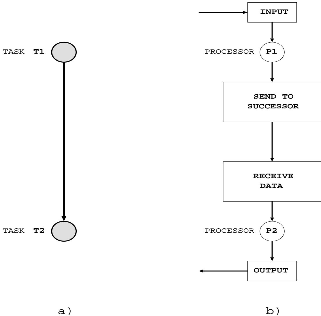
Figure 4. Message passing between connected tasks T1 and T2 which are mapped onto processors P1 and P2
